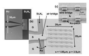
**Figure 1.** (a) SEM image of the  $5 \times 5$  PAR array with an integrated coplanar waveguide. (b) Close-up on panel (a) showing the full  $5 \times 5$  PAR array used in the experiment ( $s = 1.85 \ \mu m$ ;  $p = 3.9 \ \mu m$ ) and the air bridge connecting the coplanar waveguide to the array. (c) Individual resonators incorporating the multi-QW structure are connected by suspended Au wires of ~150 nm diameter (an array with  $p = 5 \ \mu m$  is shown in the panel).
