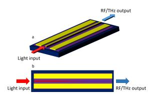
This photomixer is based on a traveling-wave (TW) photoconductor in which the pump optical wave propagates in the same direction as the generated THz wave. For the THz waves generated when the
